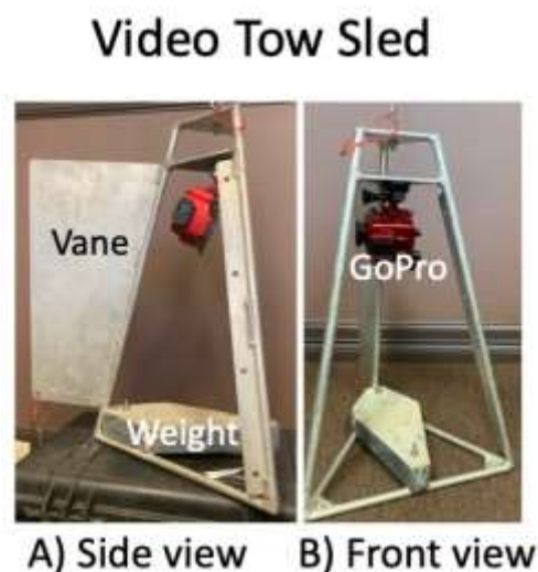
Figure 10: Towed video camera sled made of ½” aluminum rod and plate, with 25 pounds of lead bolted to the bottom, a current vane at the back, and a GoPro Hero 7 Black (set at 1440, 120 fps, 4x3 wide) in an Isotta housing rated to 200m. The camera is mounted upside down but can be angled between straight forward and 45° down.
