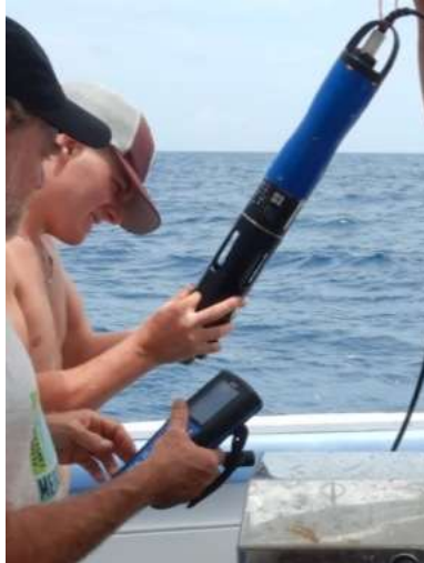
Figure 6. Deployment of the EXO3 CTD used to obtain seawater properties.
