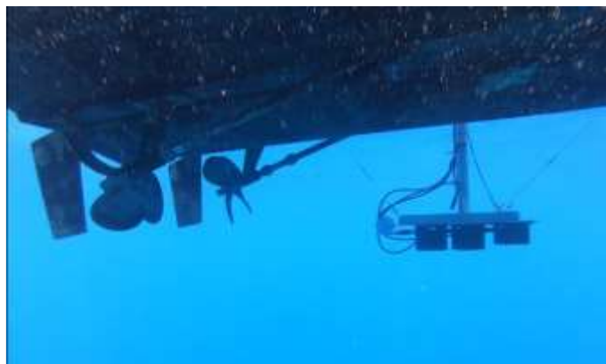
Figure 7. Echosounder transducers pole mounted over the side of a survey vessel, 1 m under the surface of the water.
